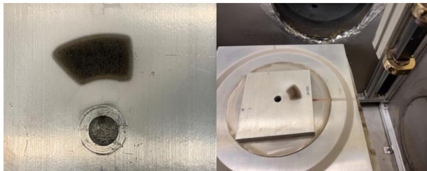
Fig 6.4 Cold-Spray Deposit of High Nitrogen Alloy on 6061 Substrate
