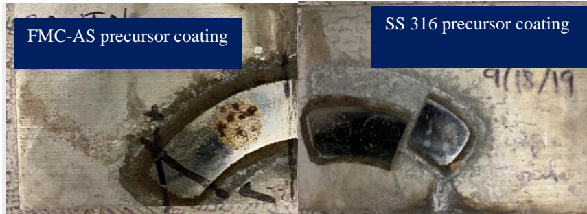
Fig 6.18 Cold-Sprayed Coating a) FMC-AS; b) SS316 on Al 6061 Substrates After a 96hrs Salt-Fog Test
