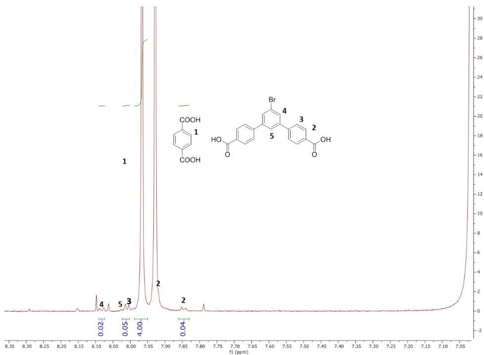
Figure S12: Aromatic region enlarged ^1\text{H} -NMR spectrum for an as prepared MOF-5-R d (A3) sample after digesting in DCI/DMSO- d 6 solution. From the integration, the molar ratio and mol% of A3 have been estimated to be 1.00:0.01 (BDC:A3) and 1 mol%.
