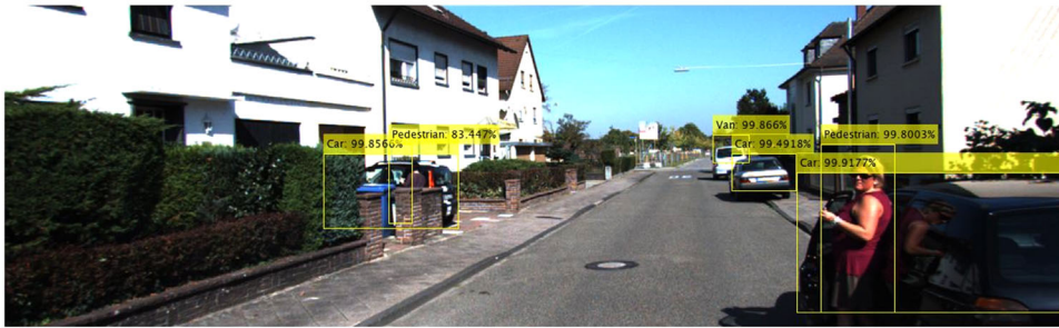
FIGURE 5 An example of the output of the YOLOv3 detector that was trained in stage 1. The objects are identified with a bounding box, with a class tag and detection confidence level shown for each object
