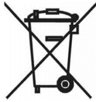
Figure 6.3: Symbol for the making of EEE. The symbol indicating separate collection for EEE consists of the crossed-out wheeled bin. The symbol must be printed visibly, legibly, and indelibly on all EEE, including solar PV modules. 108
