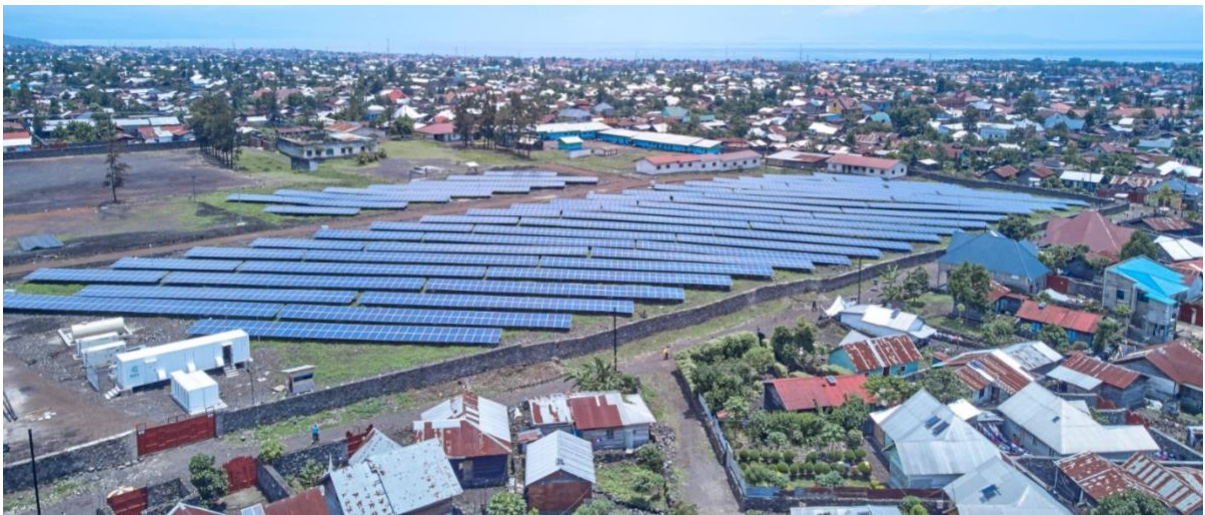
Figure 1. Aerial view of Nuru's 1.3MW solar mini-grid system in Goma
