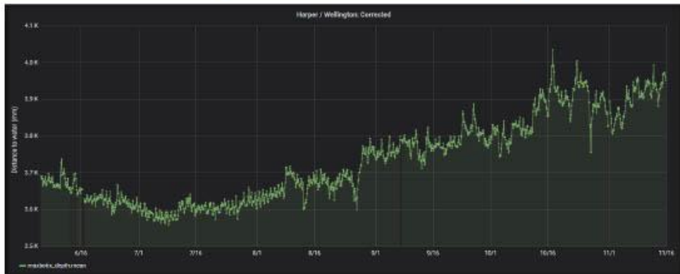
Figure 3. Real-time water level data from a sensor on the Clinton River at Harper Ave. and Wellington Cr. in Clinton Township (June - November 2020) Source: open-storm.org
