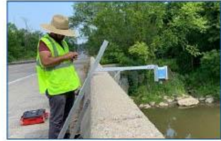
Figure 5. UM student servicing sensor node Source: UM Project Team
