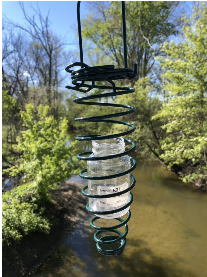
Figure 4. Corn-holder bird feeder utilized as bottle-holder for water sampling at the North Branch location in Macomb County Michigan.
