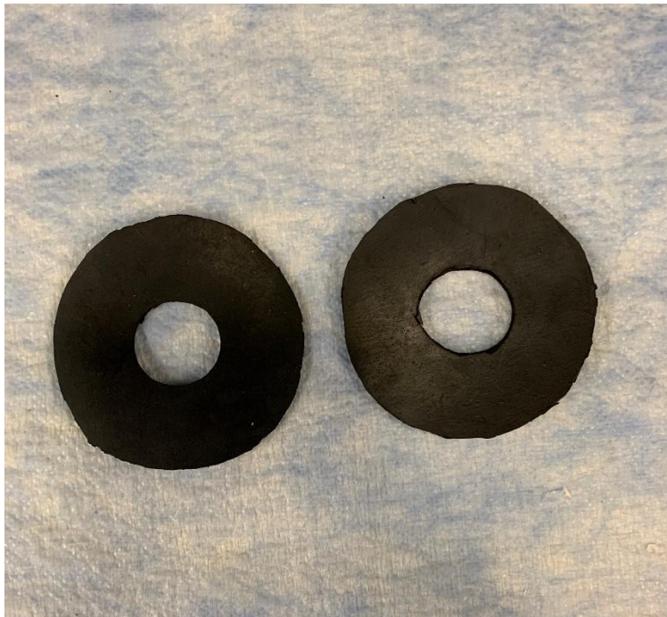
Figure 5. Sediment discs made from rubber in two sizes at 1.5 mm (left) and 2 mm (right).
