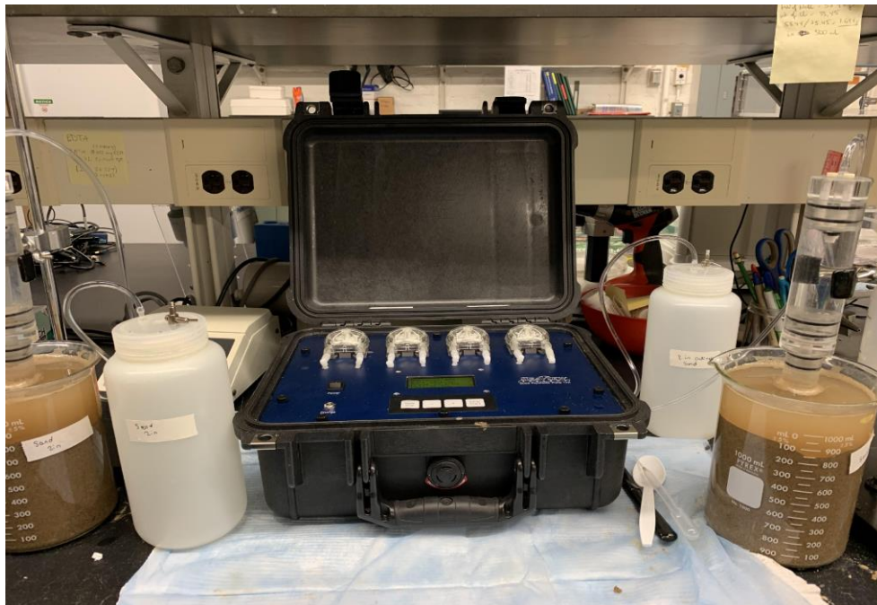
Figure 2. Porewater absorbances being tested in duplicate with iTIE 900 mLs (2 inches) from overline water in sand soil type.
