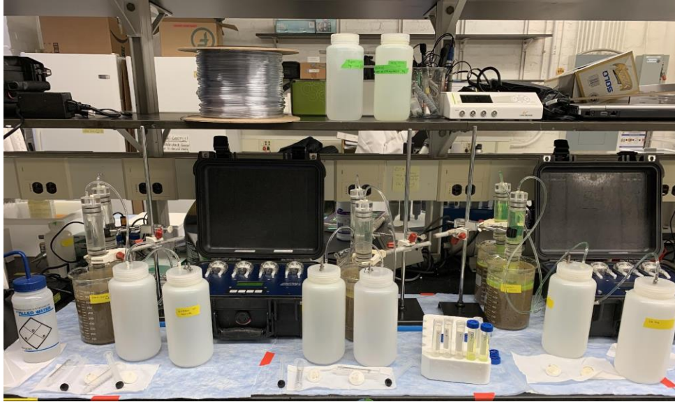
Figure 1. Green tracer dye at concentrations of 2% (5 mls of dye in 245 mls miliQ water, 0.2% (0.5 mls of dye in 249.5 mls miliQ water), and 0.02% (0.05 mls of dye in 249.95 mls miliQ water) being tested with duplicate in loamy soil type.
