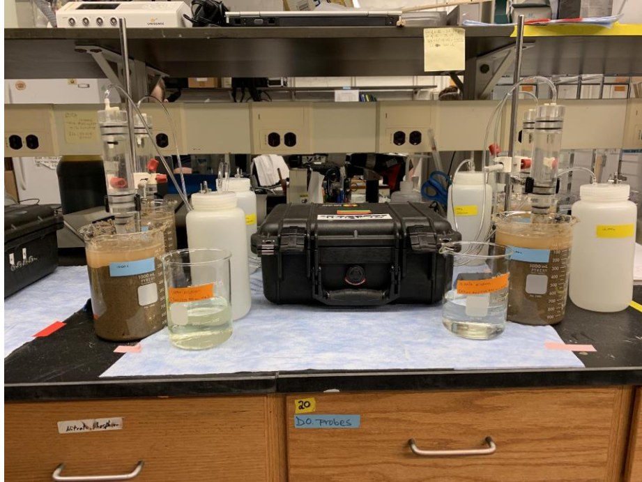
Figure 3. Green tracer dye concentrations at 0.002% (0.005 mls of dye in 249.995 mls miliQ water), and 0.0002% (0.0005 mls of dye in 249.9995 mls miliQ water) tested with duplicate in sand soil type.
