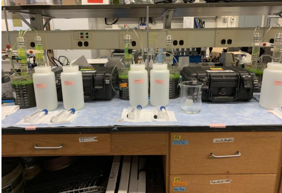
Figure 6. Display of iTIE with sediment discs, A (1.5 mm width) & B (2 mm width), being tested against control (no rubber disc) in loamy soil type.
