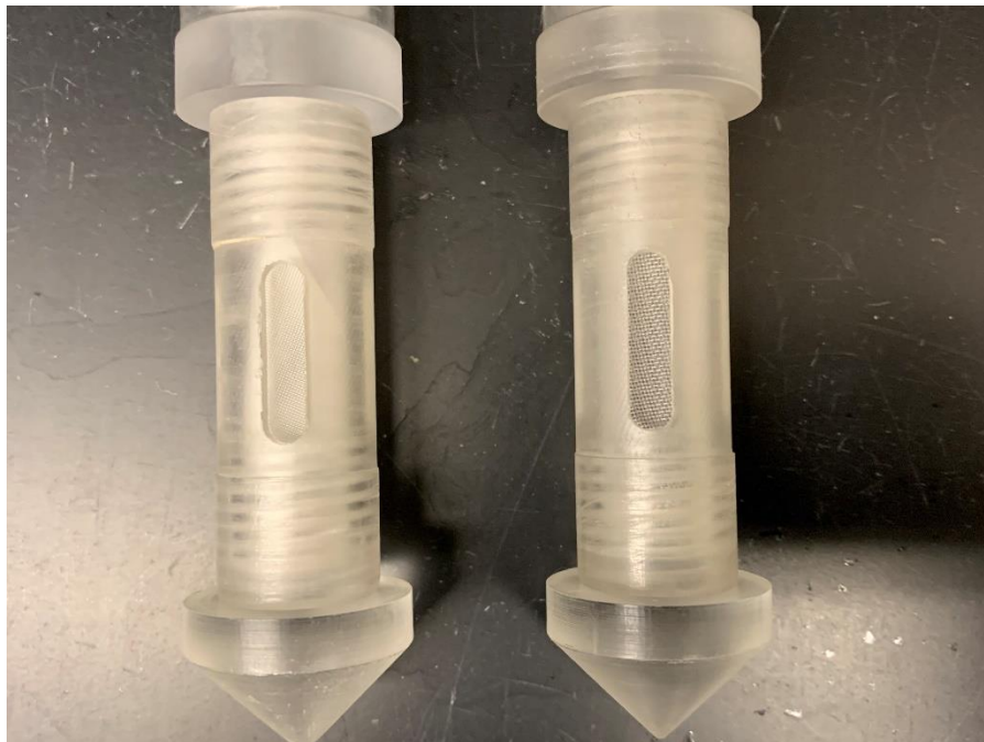
Figure 7. Display of mesh types inside iTIE porewater adapter: fine mesh (left), coarse mesh (right).
