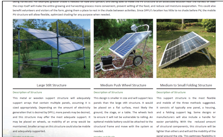
Figure 1. Example of Relative Scales of APV and PV Designs Within the Briefs. The recommended size of the PV system for each design was proportional to the relative scale of the supporting structure, as demonstrated by the various mobile PV options.
