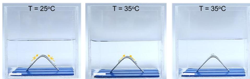
Figure S19. Heat-induced bubble sliding and merging on LCIPS. The volume of the air bubble was 10 \mu\text{L} . Scale bars, 5 mm.
