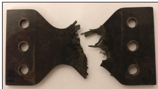
(B) Combined Tension and Shear – 45° Loading Angle
