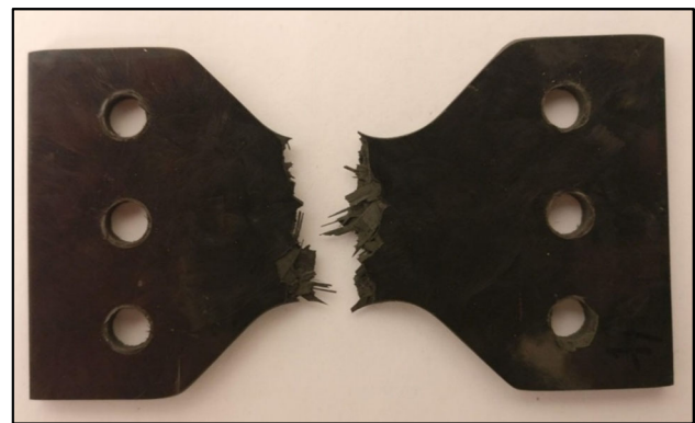
(A) Uniaxial Tension – 0° Loading Angle
