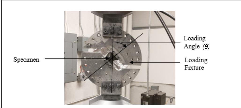
Figure 2: Modified Arcan specimen mounted on the MTS testing machine
