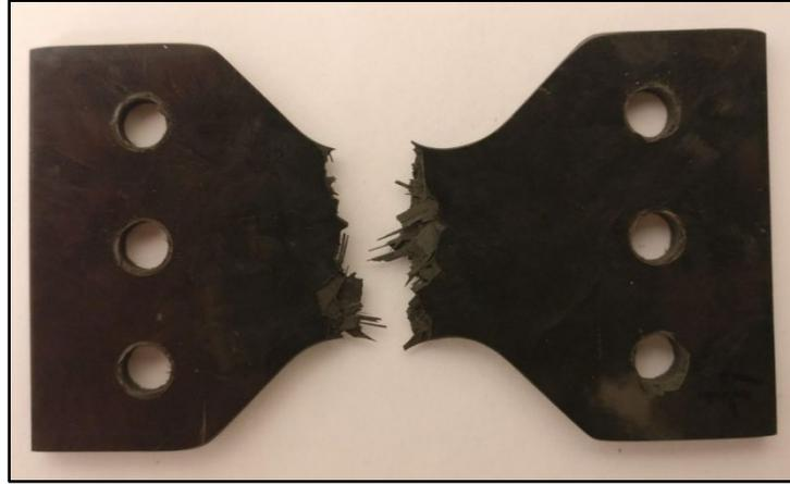
(a) Uniaxial Tension – 0° Loading Angle
