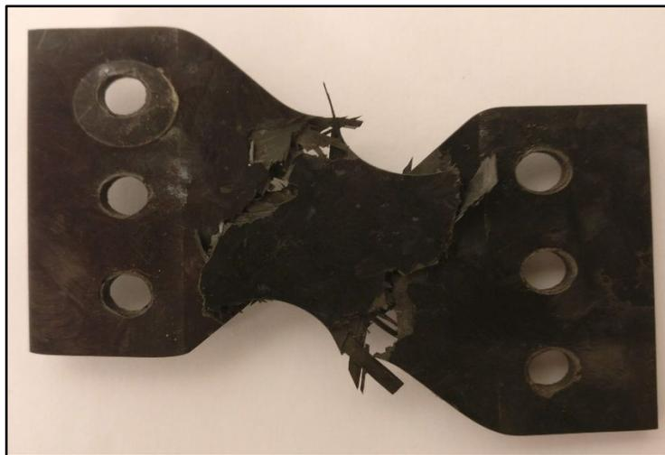
(c) Pure Shear Specimen – 90° Loading Angle
