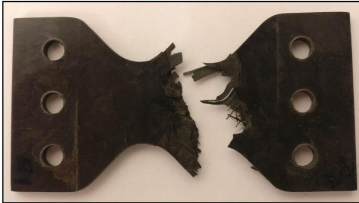
(b) Combined Tension and Shear – 45° Loading Angle
