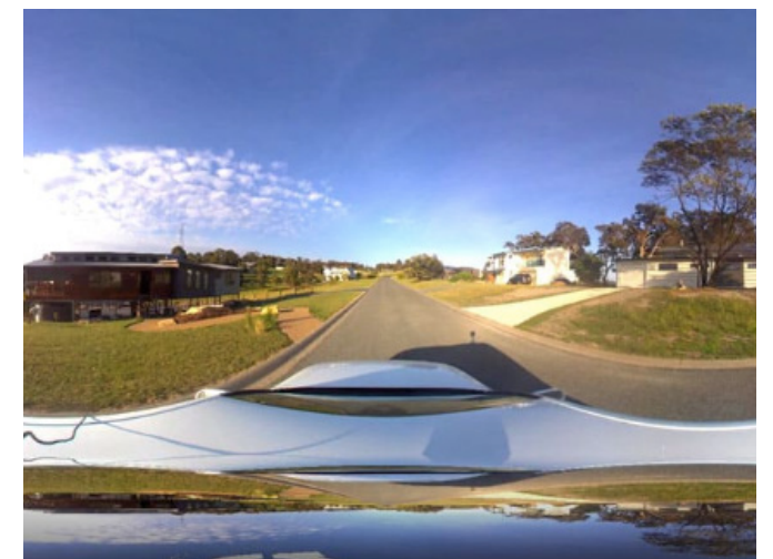
Image 2.9: Shearing Example: This picture is from the 360 imaging company NCTech's vehicle-mounted iSTAR Pulsar camera. The photo demonstrates potential distorted images for machine learning unless trained on these distortions know as shearing. Credit to GIS Lounge https://www.gislounge.com/next-generation-asset-management-with-istar-pulsar/
