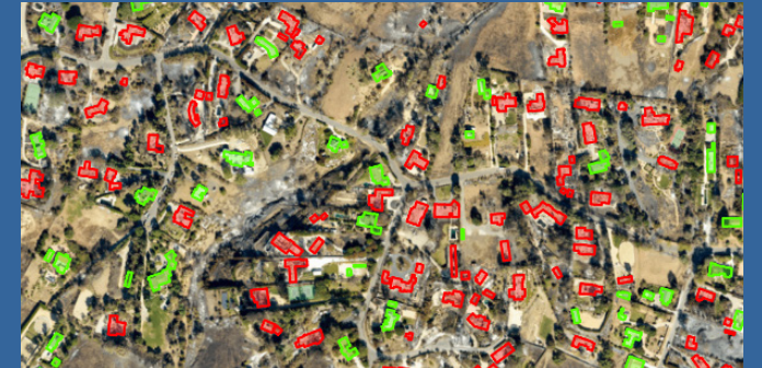
Image 3.1: Image Classification for structural damage undamaged vs. damaged classified in unique colors. Source: Esri
