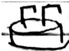
Detector uses hooks (no drill).
