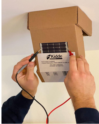
Figure 13: Solar panel power generation testing.
