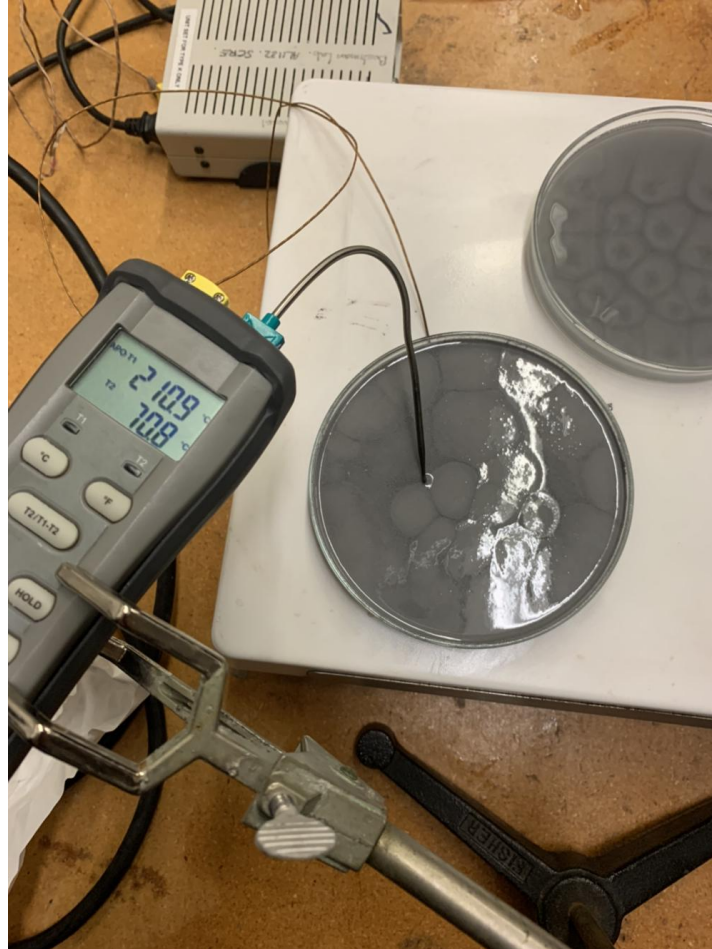
Fig. 16. Cell formation in the 1cm layer with Thermocouple data.
