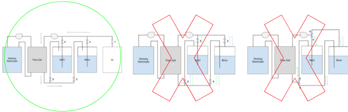
Figure 5: The above figure shows the three original systems from which our array of possible solutions were derived. The 4-valve and the 2-valve systems assumed the automated reversibility of The Kwabi Lab’s pump, which upon further inspection was not feasible under the budget offered by our sponsors. We therefore decided to focus on our four design iterations of the 5-valve system.
