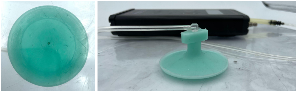
Figure 14. Static, compressed suction cup test. Left, bottom view of the compressed cup as seen through a clear acrylic surface. Right, a manometer measured the pressure within the cup.
