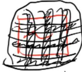
Figure 11. The mesh design is made from nitinol mesh. The mesh is heated by the surgeon and closes around the bone.
