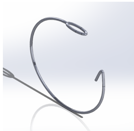
Figure 10. The “hook N’ loop” design is made from nitinol wire. The hook is threaded by a surgeon around the incus, then heated to close around the bone.
