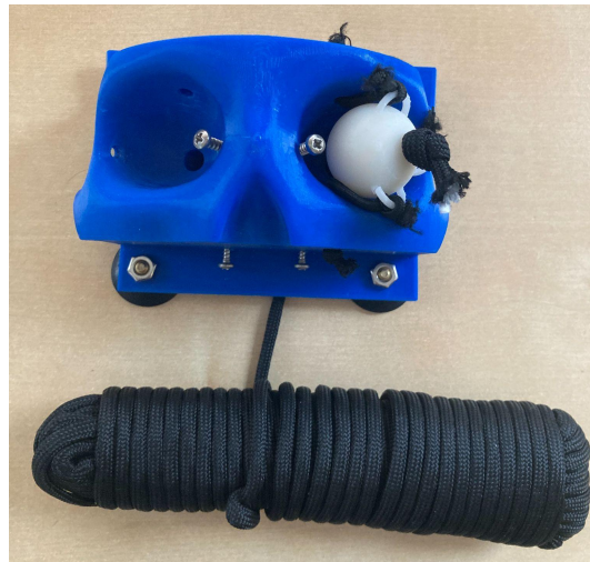
Figure 25: A picture of the built enucleation design. Elastic rope holds the three outer hooks on the eye. The polypropylene rope representing the optic nerve is threaded through the bottom of the base and 3D-printed eye. The rubber band representing the medial rectus muscle is not pictured because the hook holding it on the 3D-printed eye fractured before this picture was taken.
