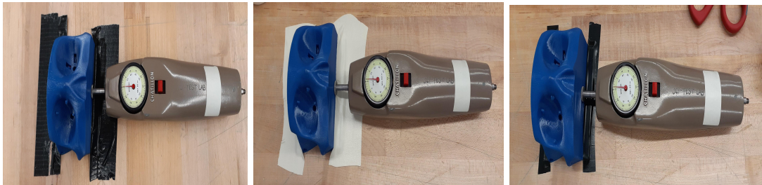
Figures 26, 27, and 28: The experimental setup for all three kinds of tape. Duct is used on the left, foam tape in the center, and electrical on the right.
