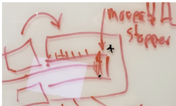
Figure 13. Hinged wire clamp concept. This combined wire holder and bender allows the user to make fine adjustments in bend length and angle by utilizing a stopper and adjustable hinge.
