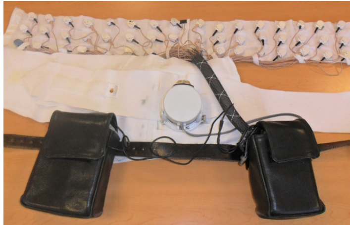
Figure 3. Vibrotactile feedback device [1] used by the Sienko Research Group in a 2013 report to look at the effect of vibrotactile feedback on postural sway. This device has a haptic display and is attached to the torso like a belt and has two battery packs.
