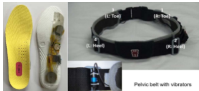
Figure B.7. This device contains foot sensors to monitor gait and is combined with a belt that provides explicit feedback at the participants waist [13]. It is also empathy based, as the researcher receives the same waist feedback while also receiving foot feedback corresponding to the participants gait.
