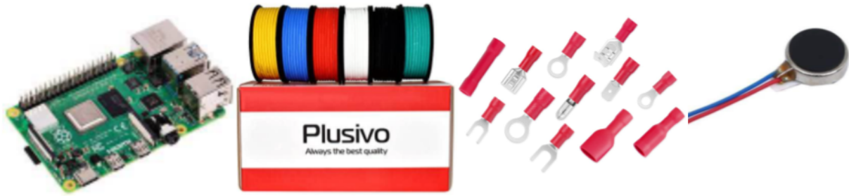
Figure 27. Wiring connection flow chart, from left to right you have the Raspberry Pi, through wiring from Plusivo, then to the wire connectors, and finally the coin motors, INEED C0820BE03L27, are crimped onto the wire connectors.
