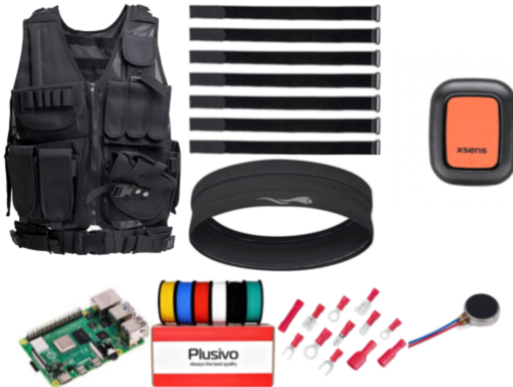
Figure 38: This figure shows most of the components that were used in our final design. We used an adjustable vest, straps and headband, as well as Xsens Dots, a Raspberry Pi, and coin motors to make our device.
