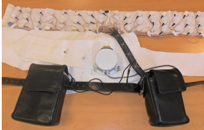
Figure B.6. The vibrotactile feedback device used by the Sienko Research Group in a 2013 report on the effect of vibrotactile feedback on postural sway [1]. This device has tactors and sensors located on the waist and was used as a proof of concept for explicit vibrotactile feedback.
