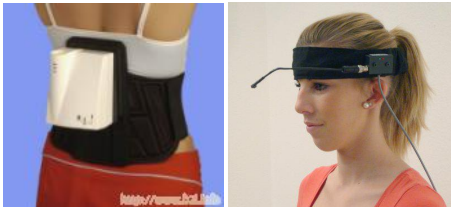
Figure B.2. Sway Star/Balance Freedom [9] is a combination of a tool to measure a patient's balance and gait, sway star, along with a vibrotactile and audio feedback device, balance freedom. Seen on the right is the Sway Star device that is used to examine the gait patterns and detect irregularities. This system is then hooked to the Balance Freedom system, seen on the right, which can provide both audio and vibrotactile feedback.
