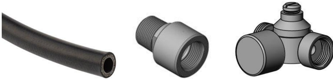
Figure 24: Recharging Hose (Left), NPT Threaded Port (Center) and Pressure Regulator (Right) CAD Drawing
