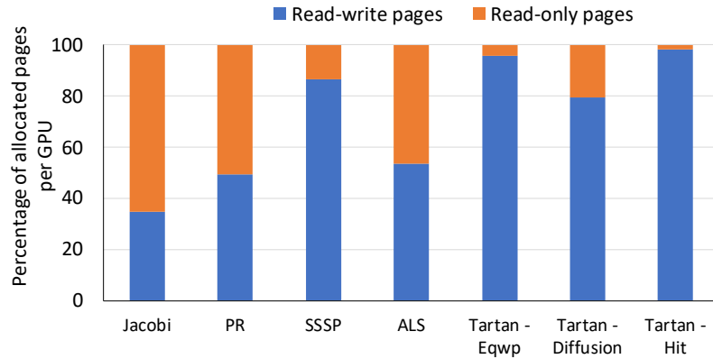
(a) Percentage of application pages that are read-write and read-only. The read-write pages are allocated as GPS pages.
