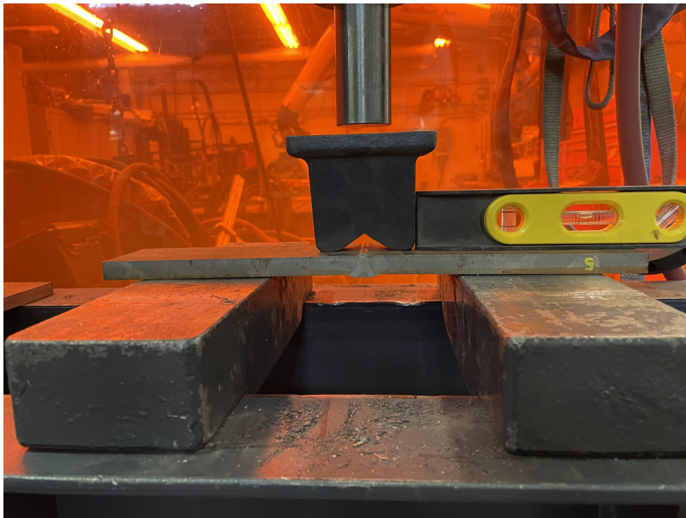
Figure 7.2: A successfully flattened specimen
