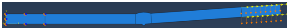
Figure 4.3: Clamping and Loading Conditions on a strip sample. Boundary conditions are in orange and blue while concentrated loads conditions are in yellow.
