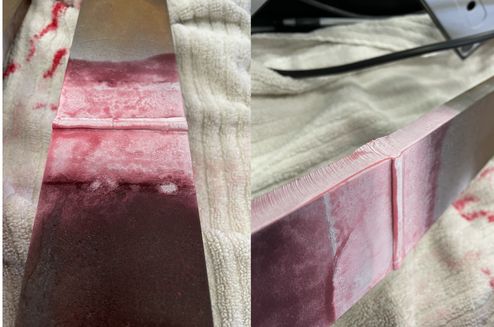
Figure 7.7: Dye penetrant testing for Test G before (left) and after (right) letting the developer sit. Note that there does not appear to be any obvious cracks at the root in either photo as expected for dye penetrant tests.
