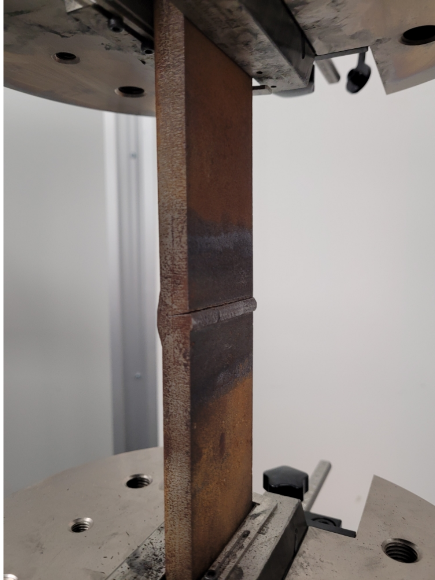
Figure 7.5: Root cracking in a plate specimen
