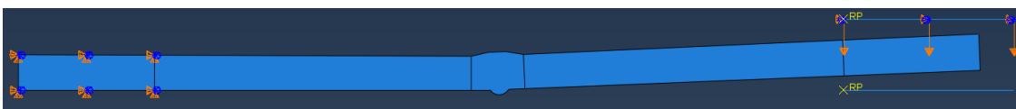
Figure 6.9: A screenshot of a two rigid clamp finite element model. The rigid body grips only need to exist as a surface, so they are modeled as just a line.
