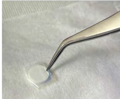
placing AEM on top of frit
