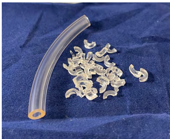
Figure A3.19 PVC tubing and PVC tubing cut up into smaller pieces
