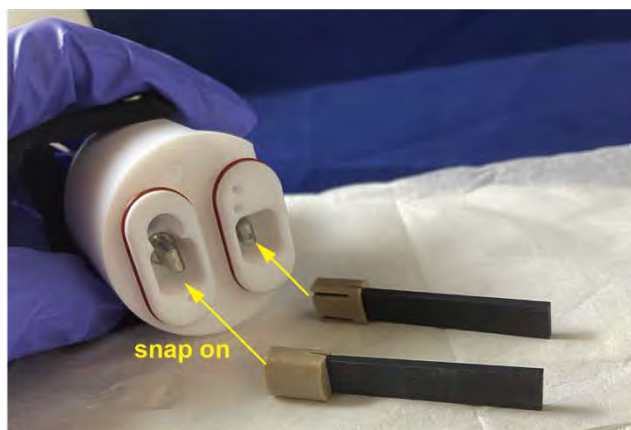
disassembled Pro-Divide cap and graphite electrodes (bottom of cap shown)
