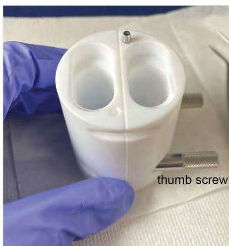
rotate thumb screws as tight as possible
