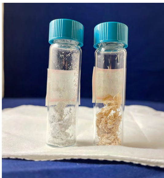
Figure A3.21 Photo of dPVC recovered from reactions performed using PVC 47k with 1 equiv. of DEHP (left) and with no DEHP (right)
