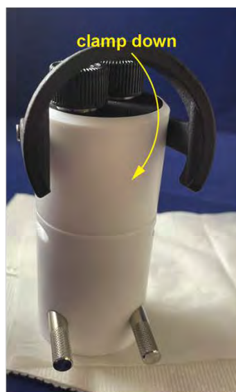
connect cap to cell but clamping down the latch
