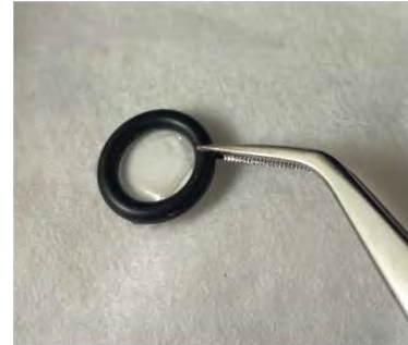
secure o-ring around frit to hold AEM in place
