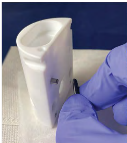
place the frit on the half-cell, the AEM should face the half-cell that will contain the polymer solution to avoid polymer clogging the frit
