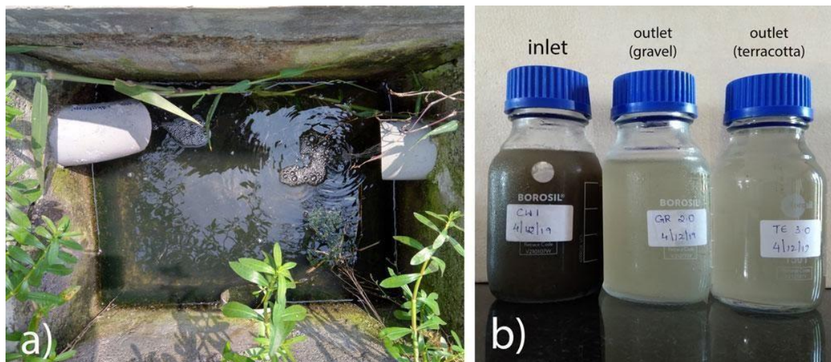
Figure 20. Outflow from gravel and terracotta setups and b) inflow and outflow samples from two setups
