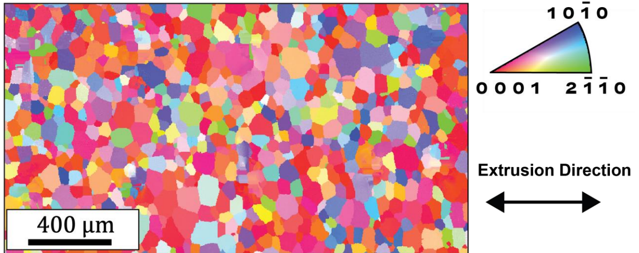
Figure 4.2 EBSD inverse pole figure map of extruded Mg-4Al (wt.%) with the average grain size of 55 μm.
