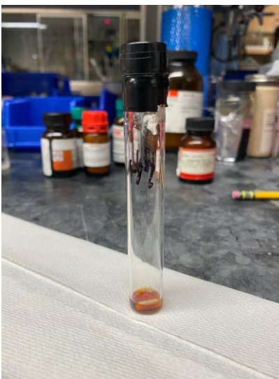
Figure 3.S4. Reaction set-up of a 0.15 mmol scale in a capped 10-mL tall vial.
