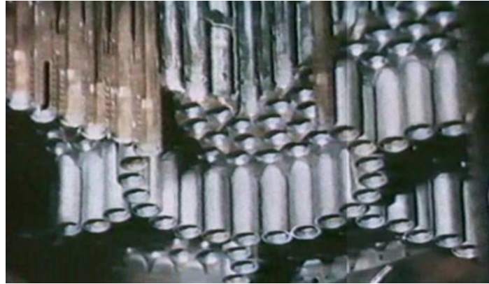
(b) Real-world geometry: hundreds of injector posts in the injector plate of a Russian RD-170 engine (Haeseler and Haidn, 2017).
