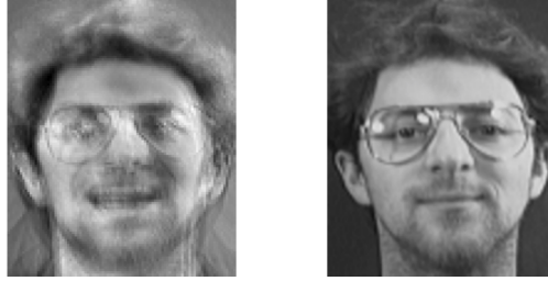
Figure 1.1: An image recovered using a model inversion attack (left) and a training set image of the victim (right). The attacker is given only the persons name and access to a facial recognition system that returns a class confidence score [1].
