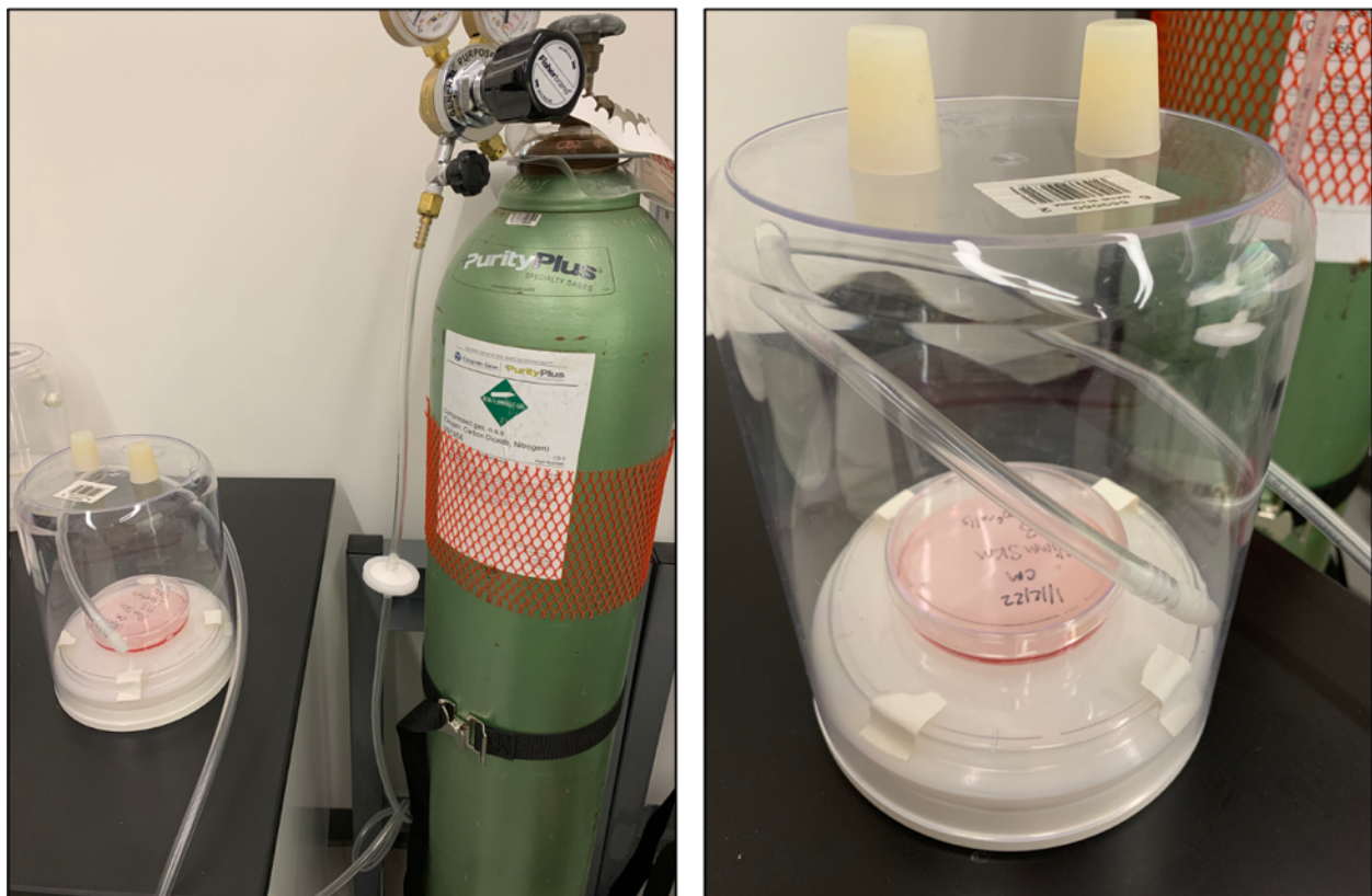
Figure 3.2 Low Oxygen Incubator Set-Up. Low O 2 gas being pumped into an air-tight chamber containing a plate of cells to displace atmospheric air. Chambers are gassed for 4 minutes prior to sealing with rubber stoppers. After gassing, cells are placed in a standard tissue culture incubator maintaining at temperature of 37 C.
