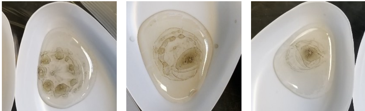
Fig. 3.62 | Topical view of PbSe colloidal solution atop EG while inside a plastic dish. These images are collected after toluene solvent has completely dried and the PbSe NCs have transitioned and/or rotated into their final spots.
