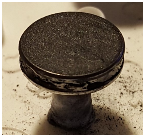
Fig. 3.4 | The top surface of an SEM holder completely coated with PbS NCs for SEM analysis.
