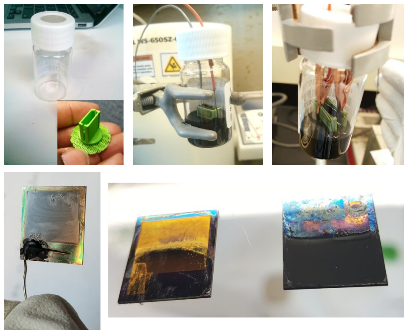
Fig. B.1 | Electrophoretic deposition (EPD) experiment. (a) Custom 3D-printed two-way Si substrate holder with 20 mL vial with septum screw cap. Two-way Si holder possessing two custom designed substrates, with each either (b) clamped with alligator clips on the ends or (c) directly attached wires via silver conductive epoxy to have positive and negative voltage to pass through substrates while submerged PbSe colloidal solution. (d) Si substrate connected to exposed end of wire via silver conductive epoxy. (e) Both Si substrates after EPD for roughly 65 hrs.
