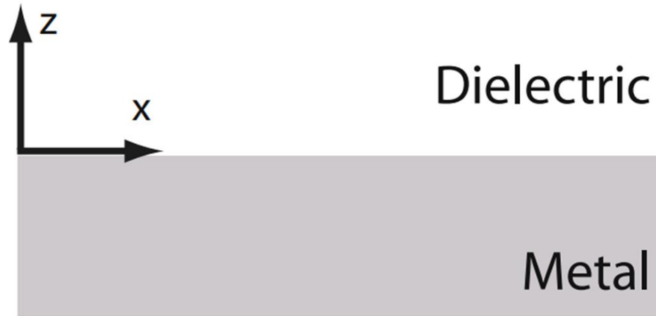
Figure 2.2 Schematic of SPP propagation along a metal/dielectric interface. An electromagnetic wave with the correct momentum constraints can couple to the interface between a metal and dielectric. The wave will propagate along this interface until it decays or reradiates. Adapted from Ref. 1
