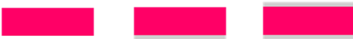
Figure S 9 Schematics of cavity and control systems. Left) a pure TDBC-PVA film deposited onto glass; Middle) a TDBC-PVA film deposited onto a 200 nm Ag mirror without a top Ag mirror. Right) a standard TDBC/PVA cavity system as described in the main text.
