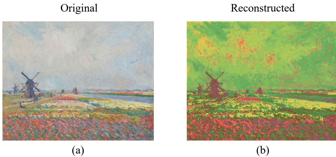
Figure 4.10: Picture reconstruction results when tuning only the dielectric layer, i.e., the fourth layer counting from the top. The average CIEDE2000 is 13.36.
