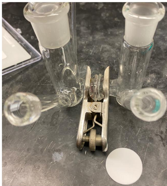
Figure B.10. Image of custom built two-compartment CPC cell constructed with an ultra-fine frit (left); a cell (right) utilizing a disposable polypropylene filter paper (shown) with 0.1-micron pore size to separate the working and counter compartments.
