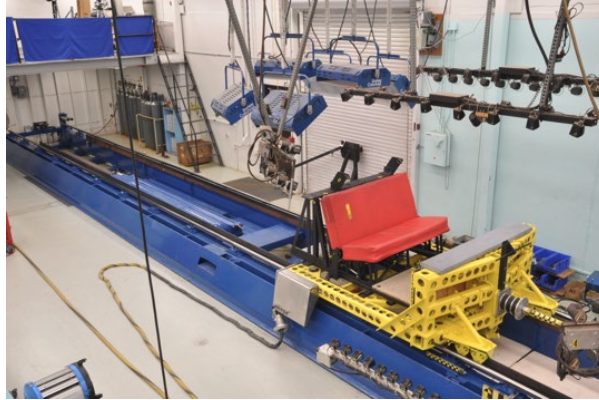
Figure 3.4. UMTRI's horizontal impact sled, shown with a child seat test buck attached.
