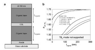
**Figure 7.** Waveguide mode analysis. (a) Device structure under calculation. (b) Effective index of  $TE_0$  mode.  $n_{glass} = 1.5$ .
