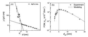
**Figure 2.** (a) Resistivity  $\rho$  of Cu-seeded Ag (Cu) film as a function of film thickness  $\underline{d}$  in log-log scale. (b) Haacke's figure-of-merit  $\overline{\phi_{TC}} (= \overline{\Gamma^{10}/R_s})$  of Cu-Ag film as a function of  $d_{\rm eff}$  where T is transmission at 550 nm wavelength and  $R_s$  is sheet resistance.
