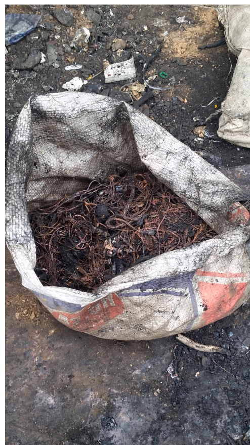
Fig. 7. A bag of copper recovered from electronic waste after burning plastic sheathing. (Source: Anne Canavati).
