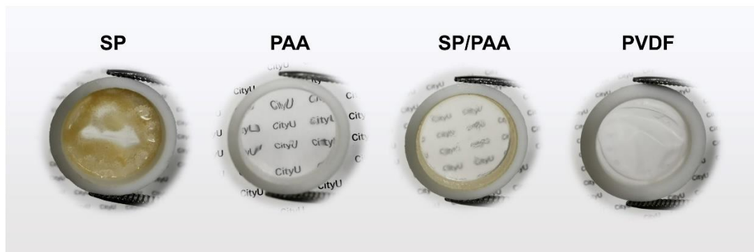
Figure S3. Photographs of the binder films. The films were obtained by dropping the binder solutions in polytetrafluoroethylene (PTFE) moulds and dried in an oven at 60 °C under air.
