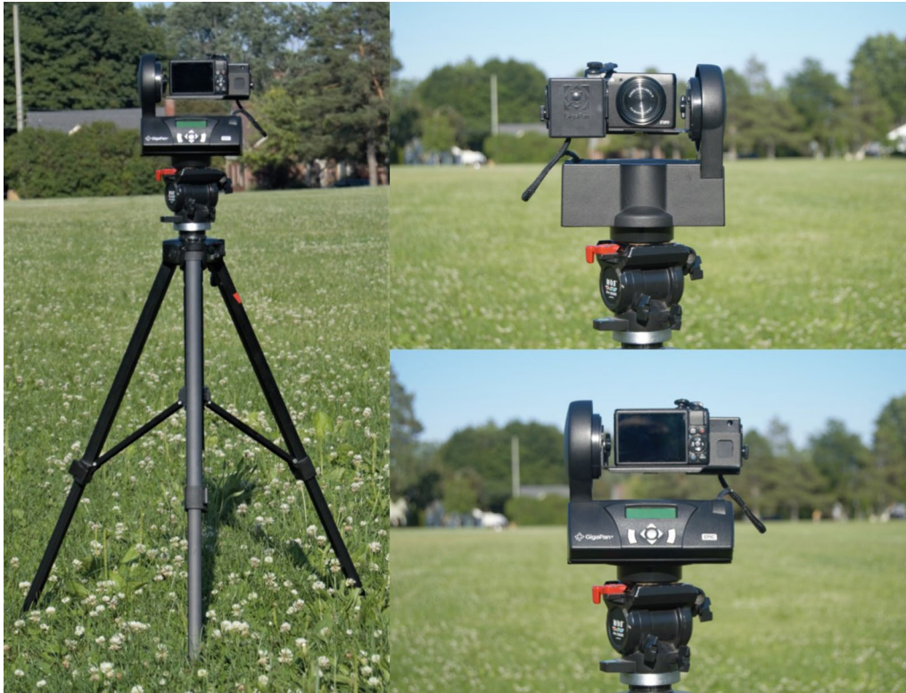
Fig. 1 Canon PowerShot® S120 camera mounted on the GigaPan® Epic and secured on a tripod
