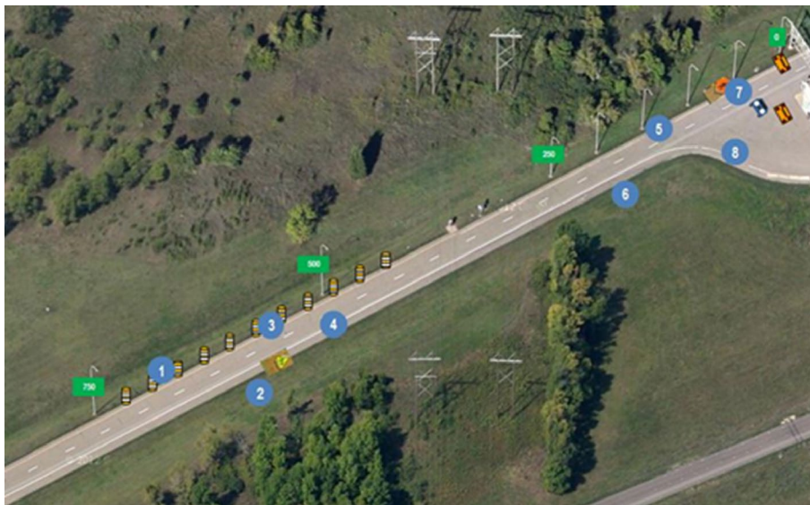
Fig. 2 Overview of the roadway scene. Each trial started at 587 meters (not indicated in the figure). The trim locations (approximately indicated by numbered circles) were at 378 m, 408 m, 426 m, 430 m, 527 m, 541 m, 565 m, and 569 m from the trial starting location. Orange construction zone barrels were located between 362 and 466 meters, an SUV faced the observer at 574 m, fluorescent road worker signs were at 411 and 561 m, and two mock fire truck rear ends were at 580 and 587 m
