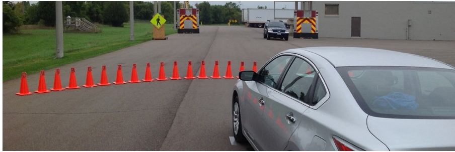
Fig. 3 Experimental set-up of study 2. Trims were presented at two angle locations, 60.19 or 77.38° from the left most cone at a distance of 30 m. Mock firetruck rear ends were located behind the trims at 54.45° and at 71.65° from the left most cone. A road sign was located at 48.72°, and an SUV at 65.92° from the left most cone
