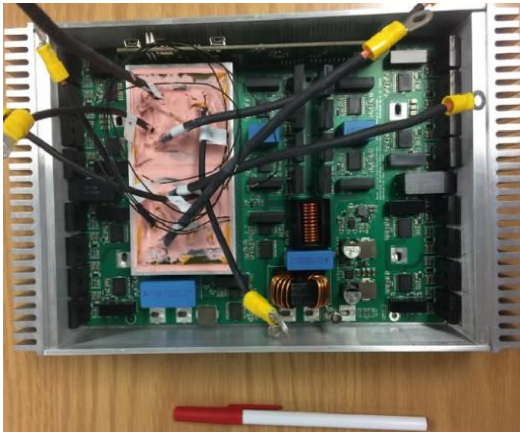
Figure 67 SiC-based DAB + transformer prototype test bench.
