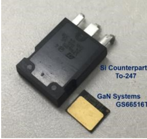
Figure 83 Leadless Top-Cooled Packaging of GaN HEMTs (GS66516T) and The equivalent circuit of the GaN+Si hybrid module
