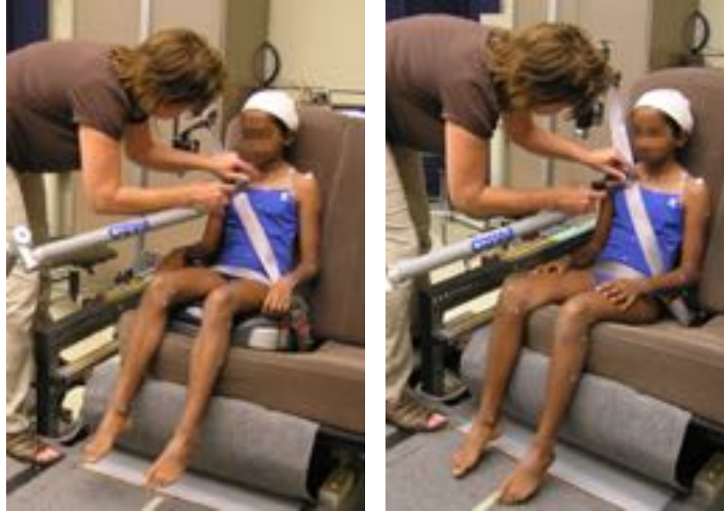
Figure 6. Investigator recording child posture and belt fit with the child seated on a booster (left) and directly on the vehicle seat (right)
