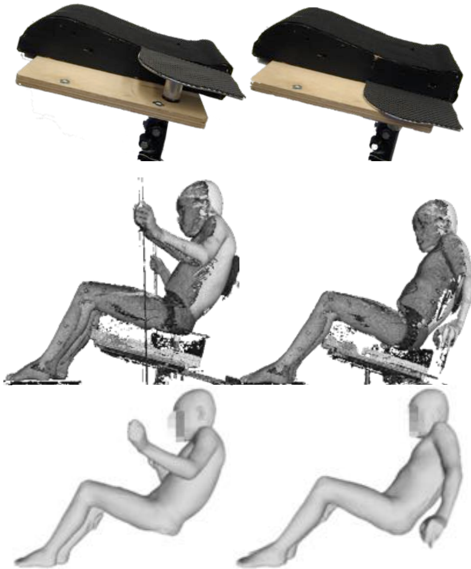
Figure 13. Booster and booster half seat (above), grayscale scans (middle) and meshes with full-body scan and hand-held scanner data merged.
