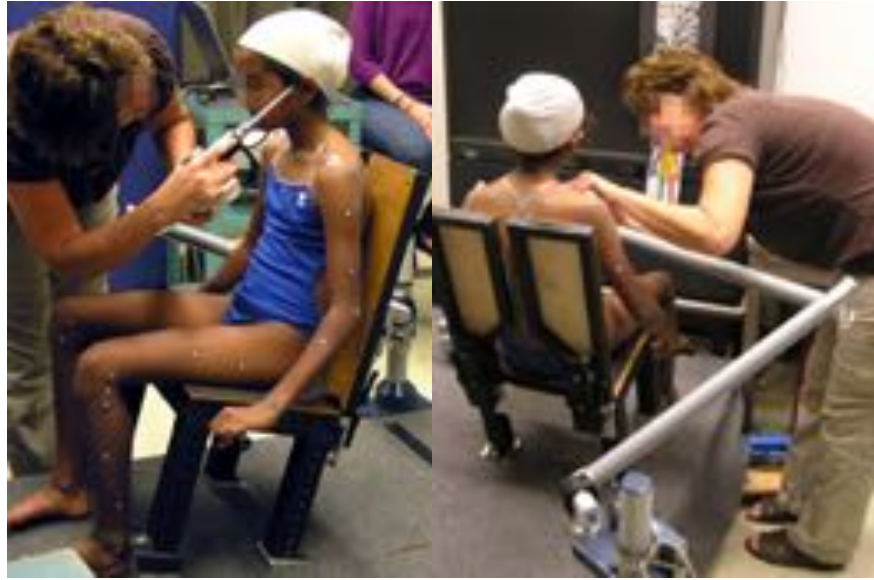
Figure 3. Laboratory hardseat used to obtain posterior and anterior body landmarks in same posture.
