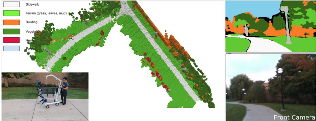
Figure 3.1: Building a semantic map for autonomous navigation. Once the transformation from LiDAR to camera is known, it is possible to fuse the LiDAR and RGB-camera information to build a 3D-map that is annotated with semantic information. The lower right shows a single camera image; its segmentation with semantic labels is shown in the upper right. Synchronized LiDAR points are mapped onto the camera image, associated to a semantic label, and then re-projected to a local frame [61] along with the semantic labels to create a 3D semantically-labeled map [50], shown in the upper left. The sidewalk is marked in white, the grass in yellow-green, and trees in dark green. In the lower left, Cassie is using the map to plan a path around the North Campus Wave Field, while staying on the sidewalk.
