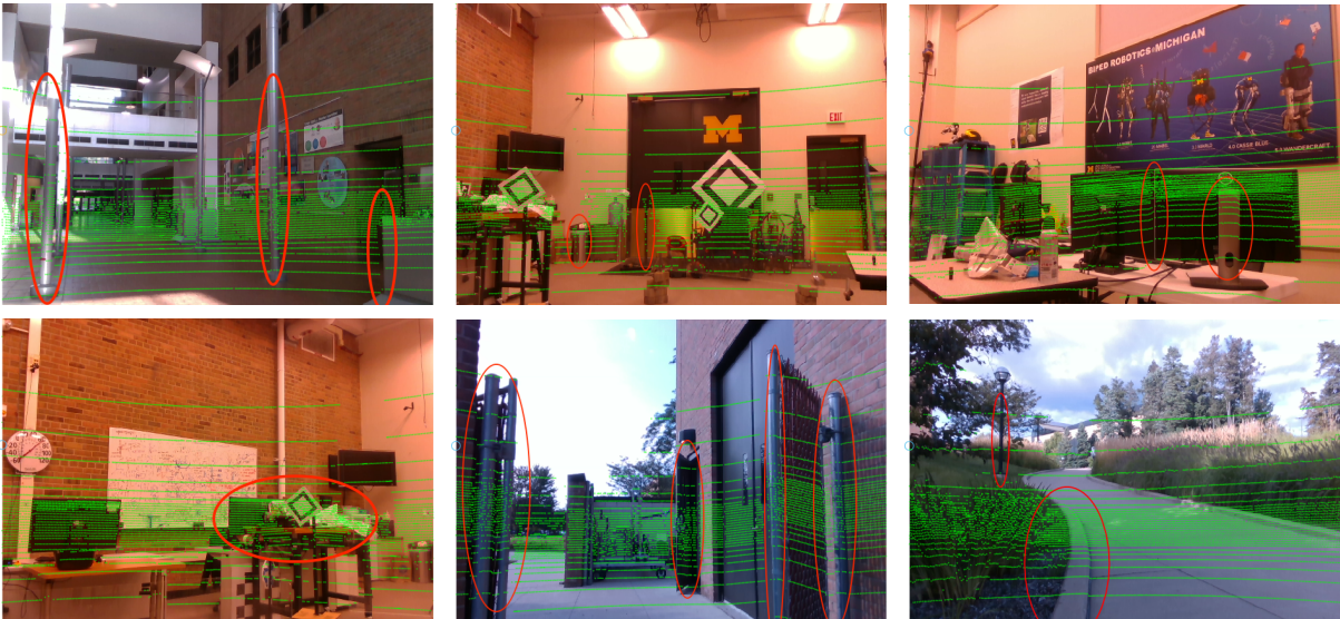
Figure 3.8: Qualitative validation results. Using the extrinsic transformation obtained by the method GL_1 applied to S_1 , the LiDAR point cloud has been projected into the image plane for the other data sets and marked in green. The red circles highlight various poles, door edges, desk legs, monitors, and sidewalk curbs where the quality of the alignment can be best judged. The reader may find other areas of interest. Enlarge in your browser for best viewing.
