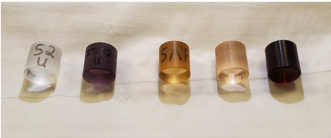
Figure 3.4: Window samples after irradiation to n-Dose 2 with total neutron fluence of 3.4 \times 10^{16} \text{ n} \cdot \text{cm}^{-2} (42 Mrad \gamma ). From left to right: S2000, I302, sapphire, BK7G18, and NBK7. The samples prior to irradiation were all as transparent as S2000 appears at left.
