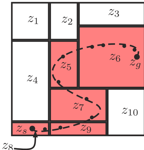
Figure 3.1: Discretized constraint space with cells z_1, \dots, z_{10} . The trajectory’s constraint values are assigned to the red cells.
