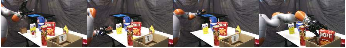
Figure 6.1: Multi-stage delivery task: place the soup in an open-top box and deliver it, then deliver the Cheez-Its to a second delivery location. To avoid spills, a pose constraint is enforced while the soup is being delivered in the open-top box.
