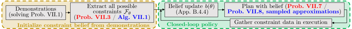
Figure 7.1: Overall method flow for adaptive planning from demonstrations. We refer to both the ideal (red), but intractable, subproblems, as well as the tractable (blue) variants of those subproblems.
