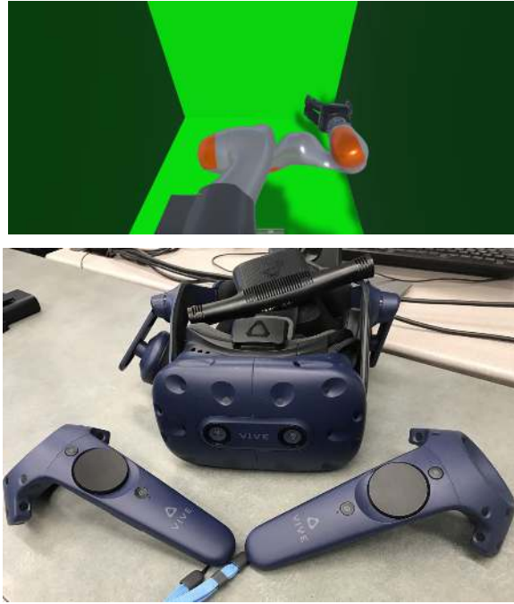
Figure A.7: VR setup. Top: VR environment as viewed from the Vive headset. The green box represents the position constraints on the end effector. The end effector is commanded to move by dragging it with the HTC Vive controllers ( bottom ).
