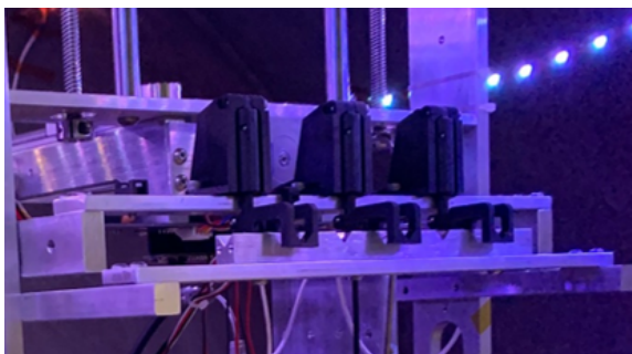
Figure 3.18: Calibration weight catcher.
