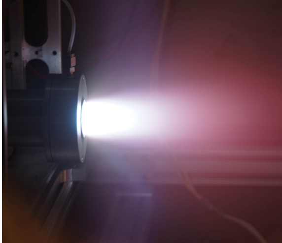
Figure 1.6: Coaxial ECR magnetic nozzle thruster firing in the Junior Vacuum Facility at the University of Michigan.
