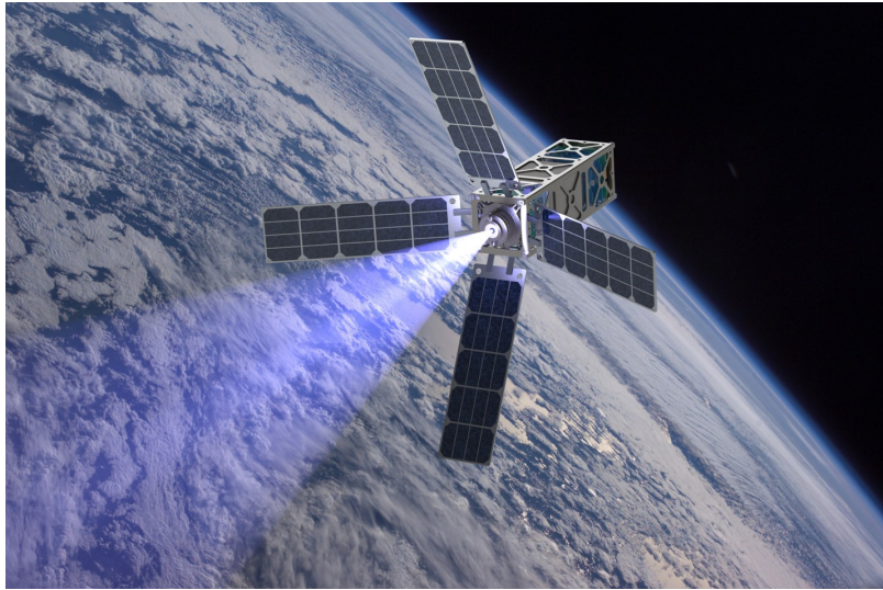
Figure 1.2: Rendering of a CubeSat with a proposed plasma thruster.
