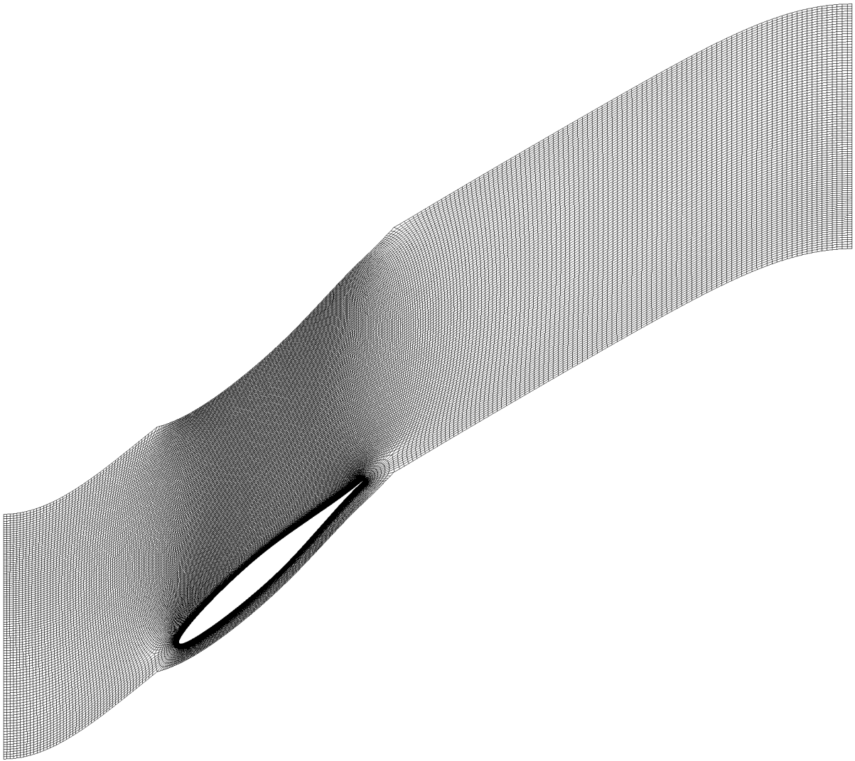
Figure 4.19: Mesh for the NACA65-010 single-stage compressor cascade case
