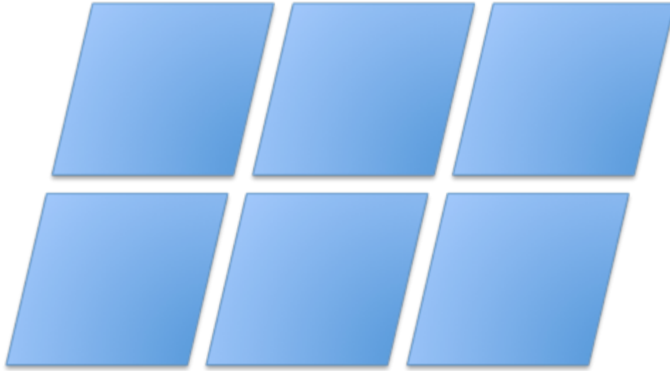
Figure 1.1 An array of rhombuses can be tiled periodically by moving copies along the horizontal and vertical directions. This unit cell is a fundamental concept in crystallography.
