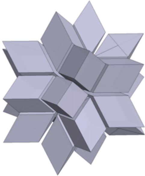
Figure 6.21: The hexecontahedron comprises twenty acute rhombohedra. Connecting the five-fold vertices will also create an internal icosahedron.
