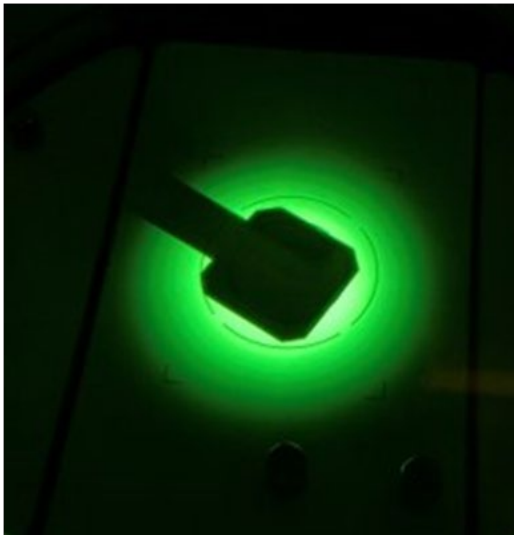
Figure 4.11 (a) Example of the Faraday cup measuring the electron beam current in the center of the beam, and (b) beam profile measured in two orthogonal directions illustrating the beam's gaussian shape with homogeneity in the center \sim 400\text{nm} .
