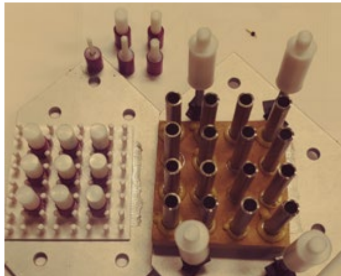
Fig. 5.49. Incoloy 4 x 4 array mockup.
