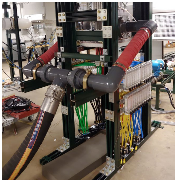
Fig. 5.15. Elephant trunk hose split into two arms connected to the test section inlet.
