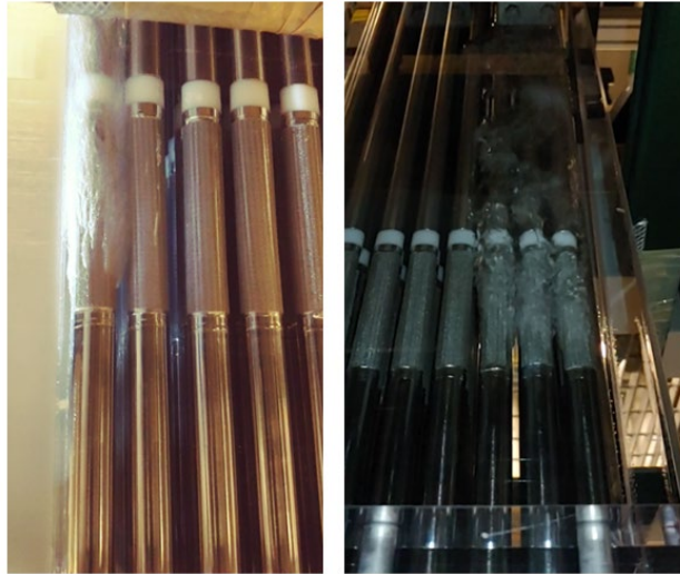
Fig. 5.25. Examples of sparging rod air injection.
